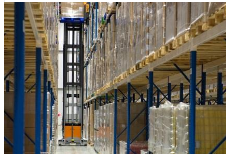
As an AS/RS (with aisle transfer)
