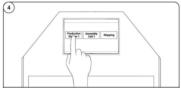
Associate taps HMIShelf screen to send robot directly to production line station or assembly cell.
